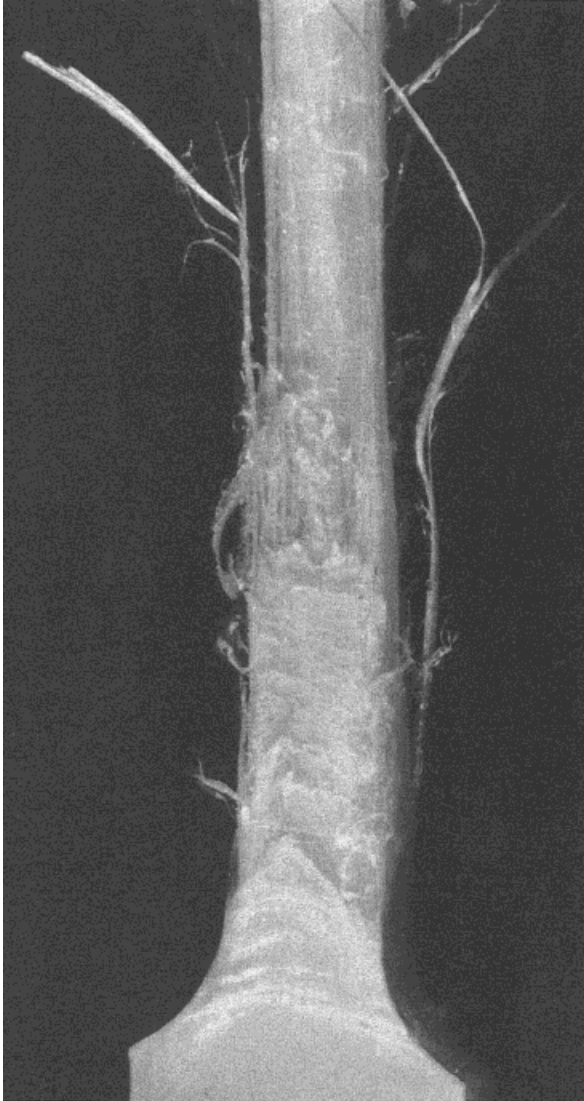
Figure 16 Microphotograph of a broken samples neck of PC/PC-PDMS 15 wt % blend. Original magnification, \times 6 .
